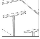
Start with ceiling, applying drywall at right angles to joists. Use panel lifter or a temporary T-brace to support weight.
