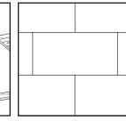
Stagger butt end (cut end) joints so joint does not extend across the ceiling. Never place a butt end next to a tapered edge. Nail or screw drywall to the joists. The GridMarX guide marks are spaced 4" apart. Use the GridMarX to gauge your nail spacing. Space nails not to exceed 7", (a minimum of 3/8" and a maximum of 1/2" from drywall edge). Screws should be spaced no more than 12" apart on ceilings.
