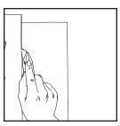
Using a straightedge and utility knife, score the drywall on the face paper side along the pencil line(s).
