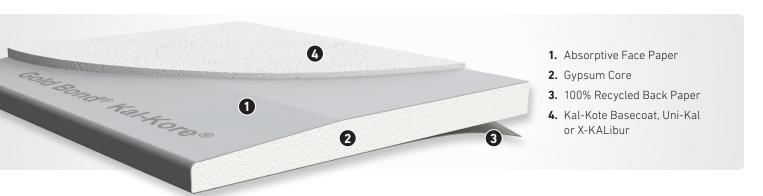
Gold Bond® Kal-Kore® Plaster Base is a tapered edge gypsum plaster base with a 100% recycled absorptive face paper surface designed to permit rapid trowel application of Gypsolite® Plaster or Two-Way Hardwall Plaster. Use Kal-Kore® Fire-Shield® Plaster Base in specific fire-rated assemblies.
