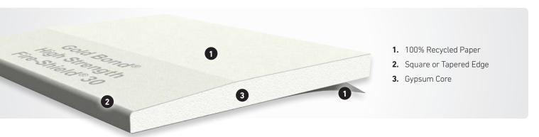
Use it for interior, 30-minute fire-rated and 1-hour fire-rated wall applications or non-rated ceiling applications. Gold Bond® High Strength Fire-Shield 30® has a fire-resistant, non-Type X gypsum core. This gypsum board is 30% lighter in weight than standard 5/8" (15.9 mm) Type X gypsum board.
