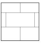
Stagger butt end (cut end) joints so joint does not extend across the ceiling. Never place a butt end next to a tapered edge.
