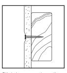
Slightly recess the nail or screw head. Indent face paper without tearing it.
