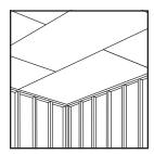
Align all electrical outlets, heating ducts, etc., so they will be flush with the drywall surface.
