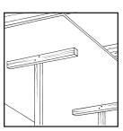
Start with ceiling, applying drywall at right angles to joists. Use panel lifter or a temporary T-brace to support weight.
