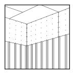
Hold the lower sidewall panel snugly against upper panel. A panel lifter (as shown) will help hold the panel until fastened. Begin fastening near the center of board and proceed to the outside.
